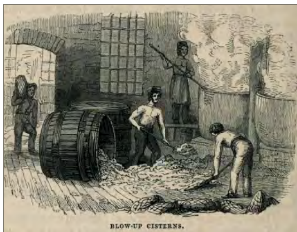
Figure 98: Emptying the hogsheads and shovelling the muscovado into the cisterns ( The Useful Arts and Manufactures of Great Britain , 1846)
