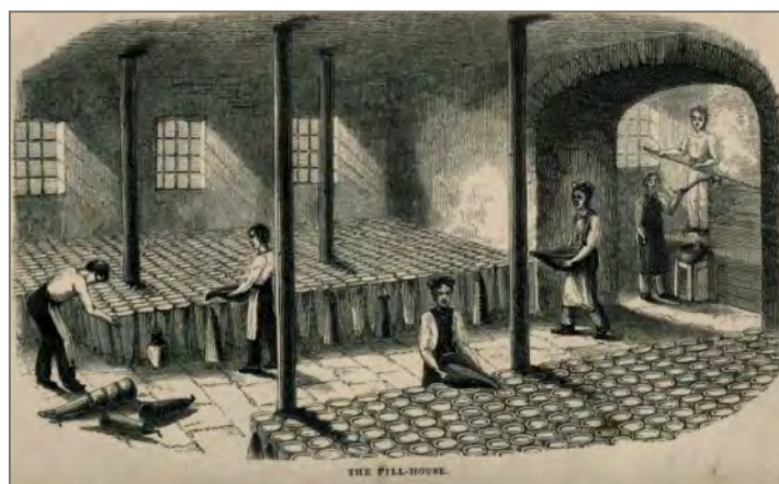
Figure 99: The fill house where the liquid sugar would be poured into conical moulds ( The Useful Arts and Manufactures of Great Britain , 1846)
